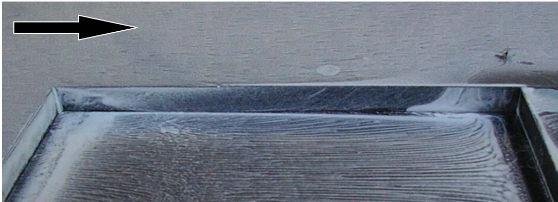
Figure 23 Upstream tandem cavity sidewall oil flow visualisation – closed type ( l/h=16 , M=0.91 )
